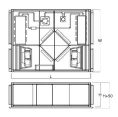
Summer operation: Outside Air 35°C K.T. 40% rH & Inside Air 25°C K.T. 50% rH (evaporation 7,2°C /Condensation 50°C) Winter operation: Outside Air 0°C K.T. 80% rH & Inside Air 22°C K.T. 40% rH (evaporation -5°C /Condensation 40°C) Electric pre-heaters must be used in case the outside weather is between -5°C and -15°C and there is condensation. In humid climates, return air channel must be insulated against condensation. With electric heater, the device's dimension extends as 300mm.
