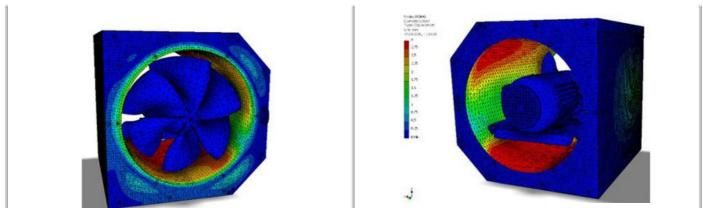
Performing structural analyses of the force that will come on the jet fan electric motor table under structural and flow loads.
