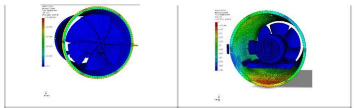
Performing structural analyses of the force that will come on the jet fan carcass structure under structural and flow loads.
