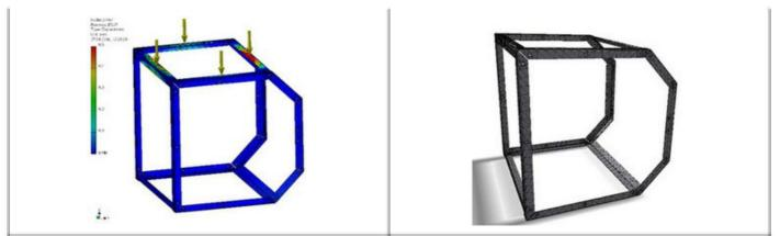
Performing structural analyses of the jet fan carcass structure under structural and flow loads that will come on it in the axial direction.
