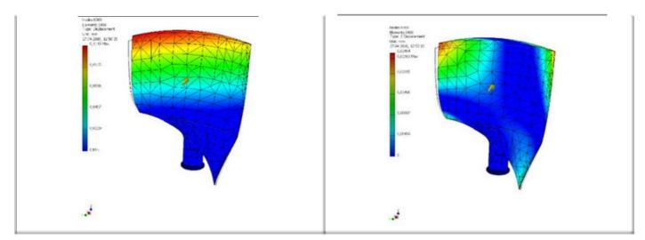
Performing static analyses under the flow and structural loads that will come over the front body used in the connection of the wings to the body.
