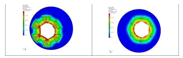
Performing stress analyses under the flow and structural loads that will come over the rear body used in the connection of the wings to the body.
